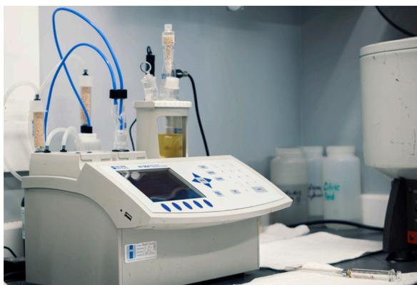
measure the amount of moisture in the incoming cooking oil and in the finished biodiesel product. The goal in biodiesel production is to have the lowest moisture content possible in the final product. If they notice the moisture content is rising, they can proactively adjust their process and ensure a consistent result. Without a
